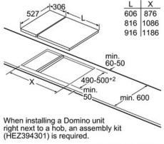
Measurements in mm
